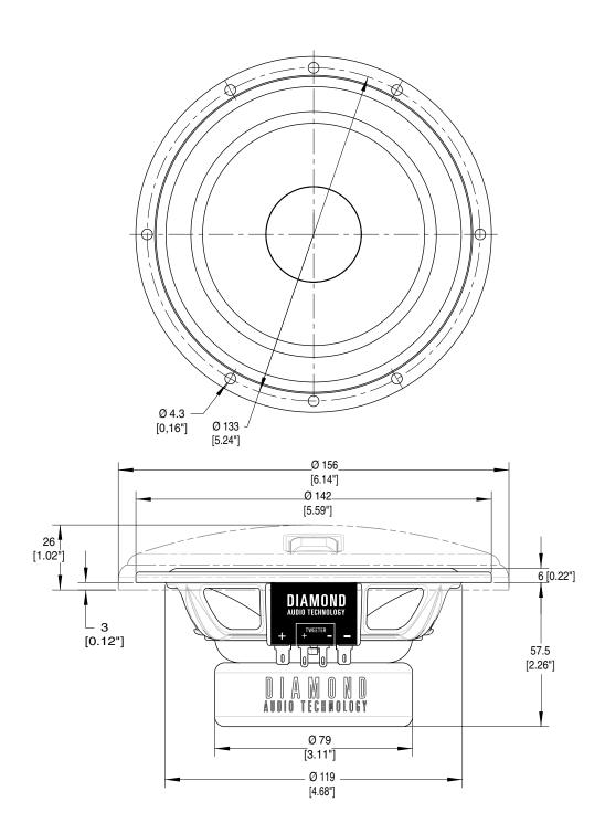
M361, M361i General dimensions in millimeters and [inches]. Not to scale.
